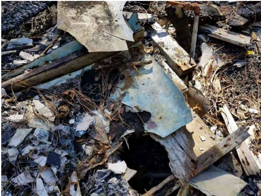
View of HA-01: Beige Sheet Flooring with Fiber Backing
