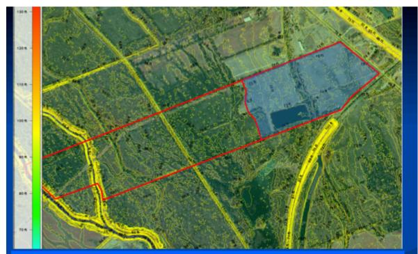
LiDAR one-foot contour map shows that the land is relatively flat and slopes gently to the southwest away from Hwy. 1. Elevations range from 75 feet at the highway to 70 feet at the rear of the proposed 50-acre site.
