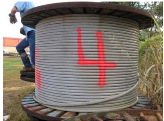
Reel #4 – 900-ACSR Wire – Approximately 4270 lbs
