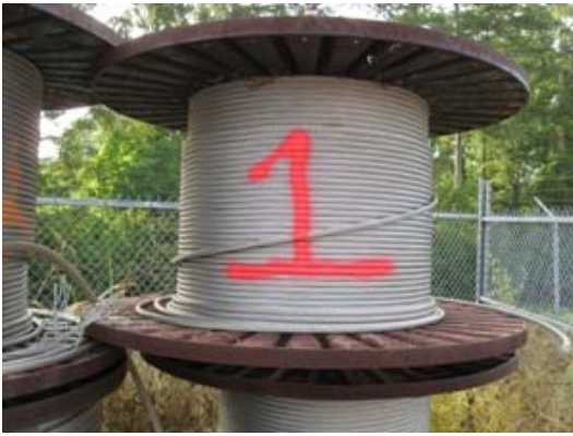
Reel #1 – 477-AAC Wire – Approximately 830 lbs
