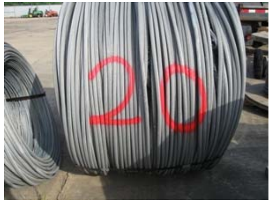
No Spool #20 – 636-AAC – Approximately 7380 lbs (Note: Steel guy wire in middle of roll)
