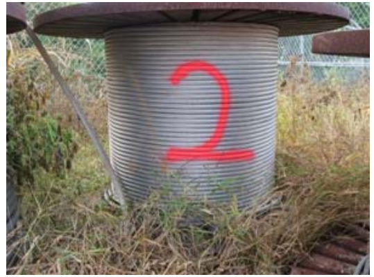
Reel #2 – 556.5-ACSR Wire – Approximately 1160 lbs
