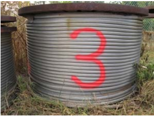
Reel #3 – 1400-ACSR Wire – Approximately 6000 lbs
